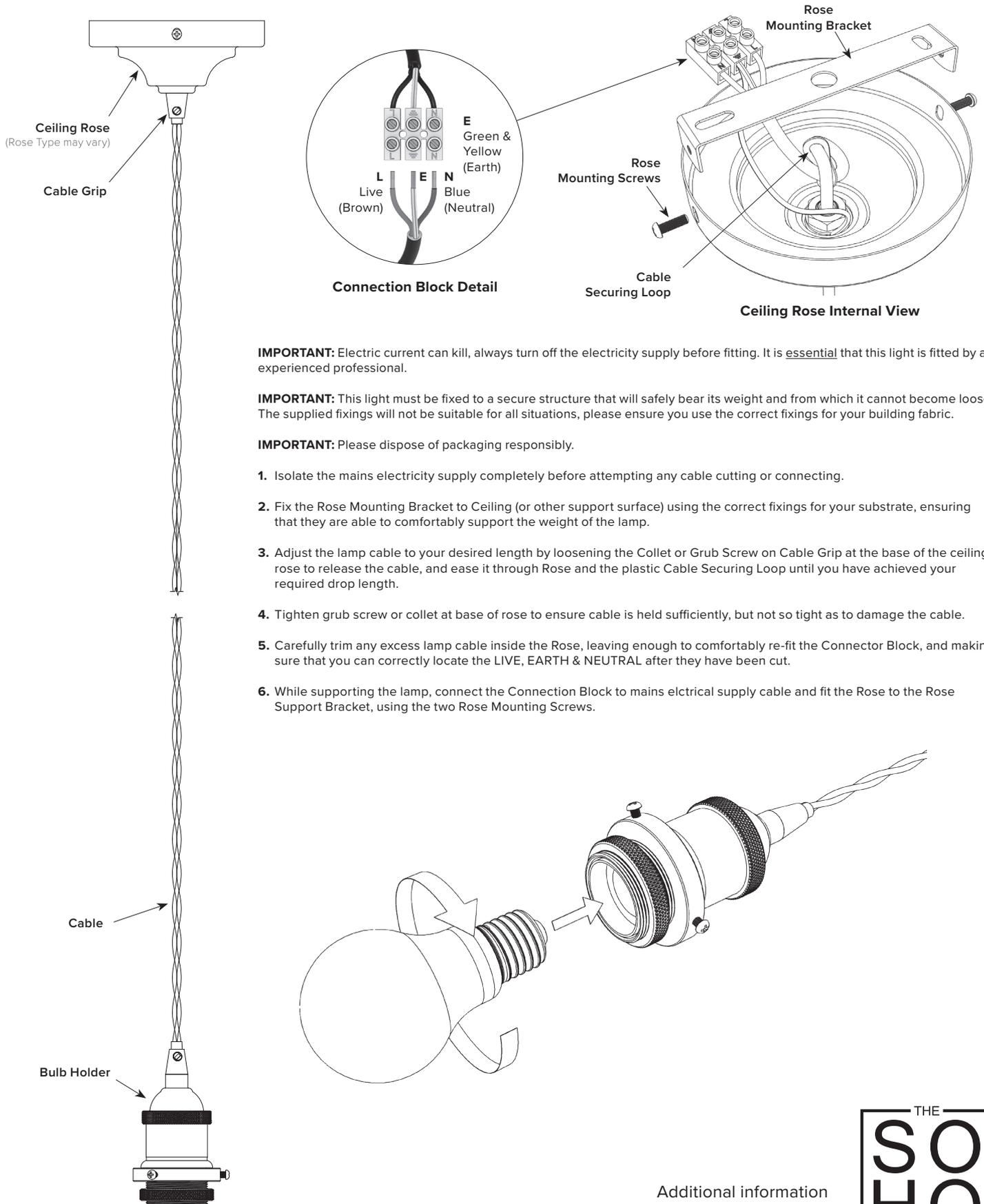
**IMPORTANT:** Electric current can kill, always turn off the electricity supply before fitting. It is essential that this light is fitted by an experienced professional.
