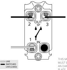
THIS MODULE MUST BE FITTED TO AN EARTHED FACE PLATE
