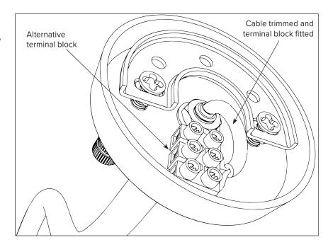
Trim the existing cable as short as possible, while still leaving enough length to strip and fit the alternative terminal block provided, this needs to fit inside the base plate. See illustration above.
