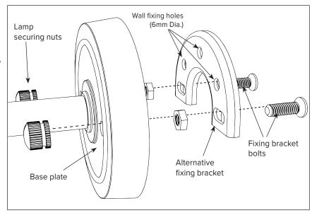
Remove bolts from the standard fixing bracket and fit them in the same configuration and spacing on the alternative, 'U' shaped bracket, use the holes in the base plate as a spacing guide. See illustration above.
