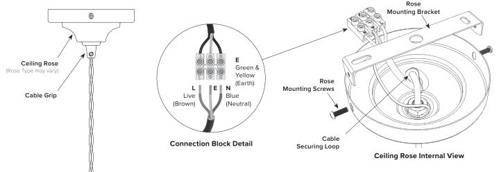
**IMPORTANT:** Electric current can kill, always turn off the electricity supply before fitting. It is <u>essential</u> that this light is fitted by an experienced professional.
